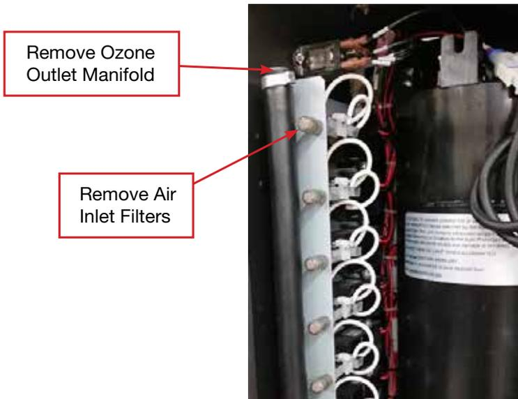
**Figure 1. Ozone Generator Assembly**
