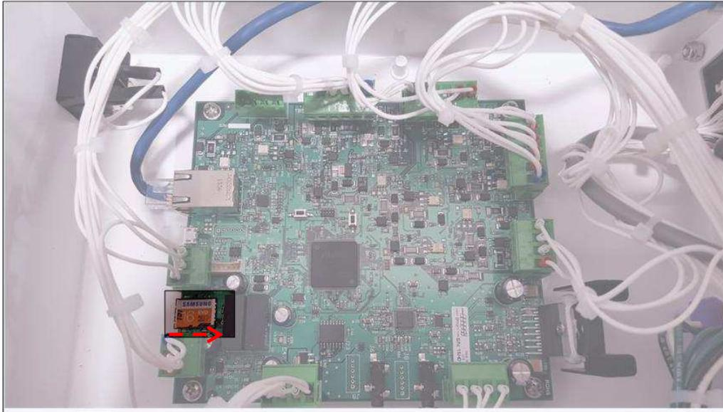
6.2. Connect the SD card to a PC, you will likely need a micro-SD to SD card adapter. Check inside the frame for a plastic sleeve, the adapters are now provided with each unit inside this sleeve
